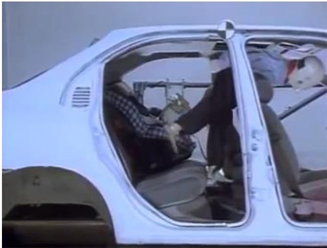
Figure 4: Capture taken from a crash test video of a frontal impact with an unbelted child crash test dummy in the rear seat. 15
