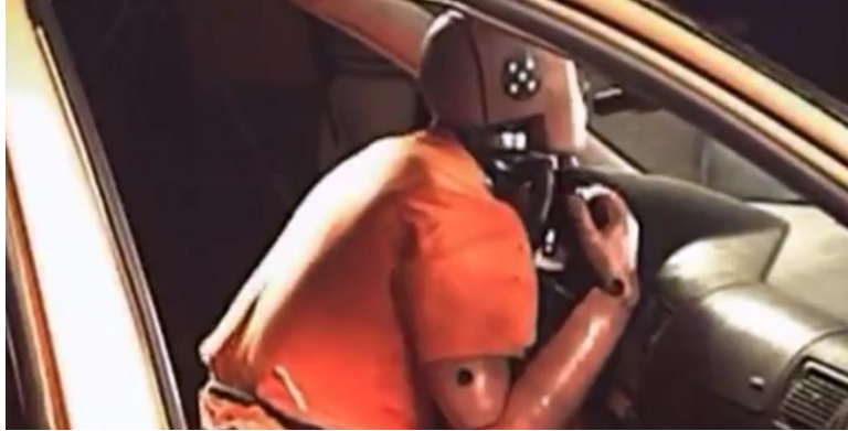
Figure 3: Unbelted crash test dummy during a 30 km/h impact.
