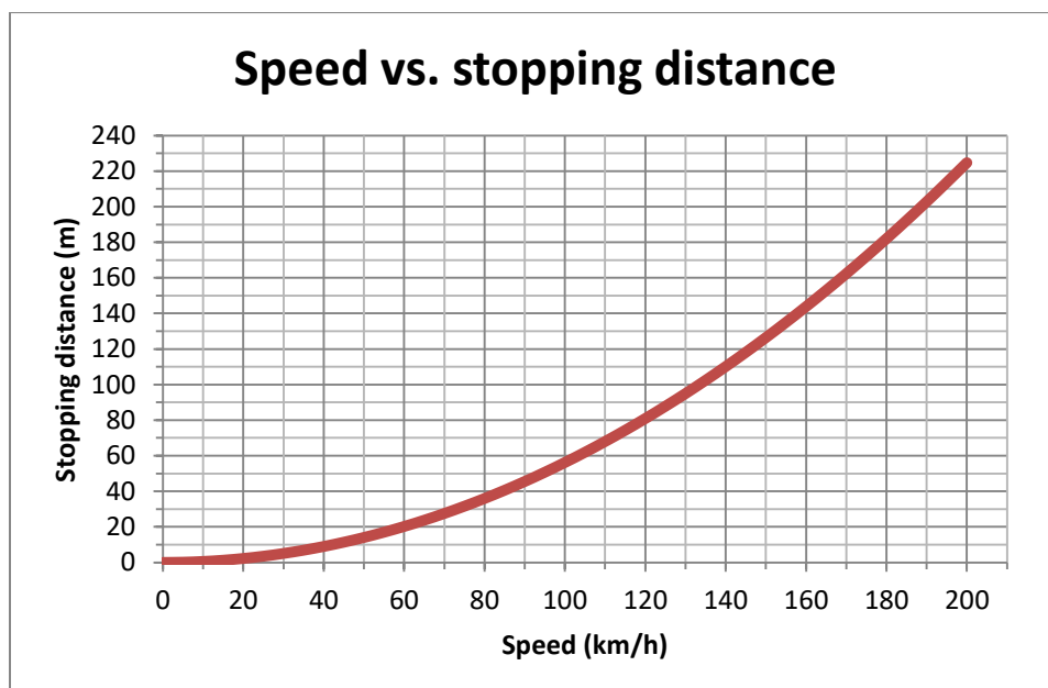
Figure 1: Graph of the exponential relationship between speed and stopping distance. Given the same braking rate, if the speed is doubled, the stopping distance is quadrupled. If the braking rate is changed, the specific distances will change, but the relationship remains the same.
