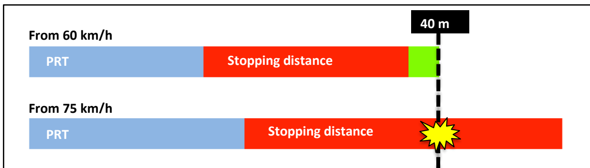
Figure 2: Illustration of the distance a vehicle would travel during a 1 second perception-response time, and the distance required to brake to a stop from 60 km/h and 75 km/h. If both vehicles are initially 40 metres away from a hazard (i.e. left-turning vehicle), the vehicle initially travelling at 60 km/h would brake to a stop 3 metres before reaching the hazard, while the vehicle initially travelling at 75 km/h vehicle would crash into it, with 12 additional metres required to stop.
